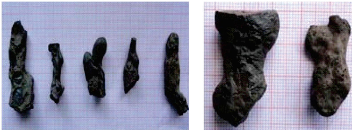
Figure 10: Fritter/waste iron from Iron workshop, PLN
